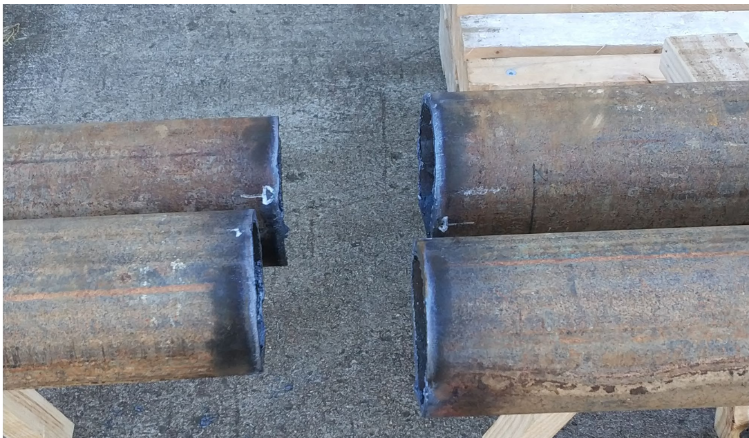
Figure 7: Caroline-1 5-1/2" Casing Cut with Oxy Cutter
