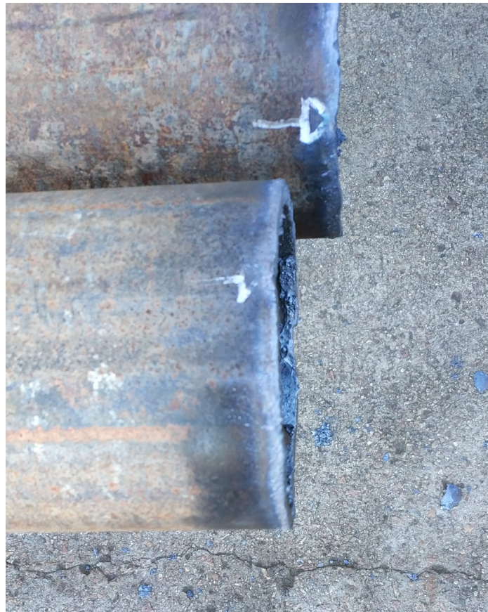
Figure 7: Caroline-1 5-1/2" Casing Cut with Oxy Cutter
