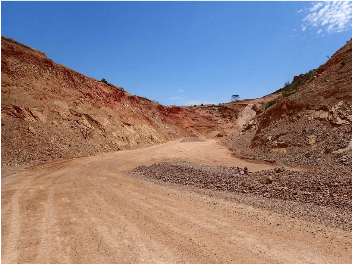
Northern quartzite pit looking north. Minimum floor level is at 183.7 mAHD, 13 m below adjacent drainage line. Floor elevations measured by unmanned aerial vehicle survey (UAV) and accessed via Propeller (2020).
