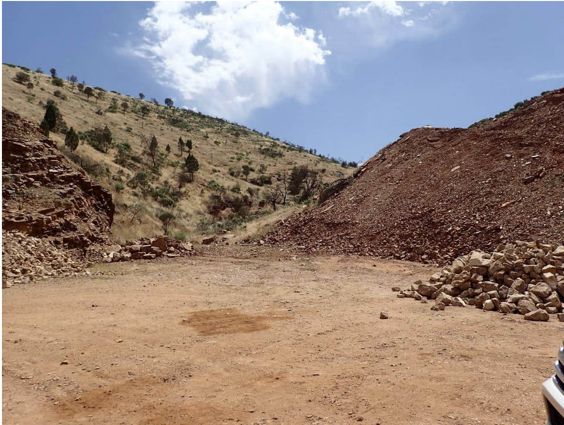
Eastern Dolomitic Pit looking west – Pit floor is at relative level of 213 mAHD. Floor level measured by unmanned aerial vehicle survey (UAV) and accessed via Propeller (2020).
