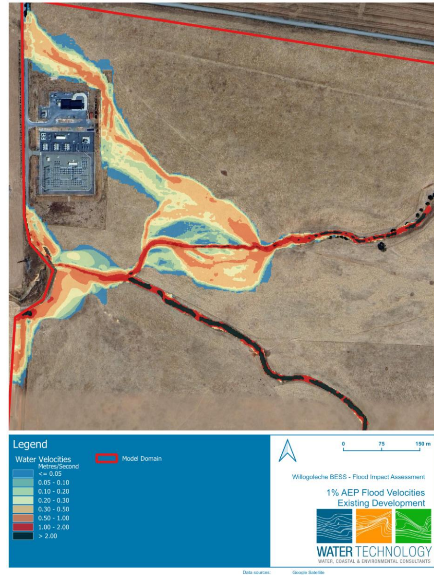
Figure 2-5 1% AEP Velocities Existing Conditions
