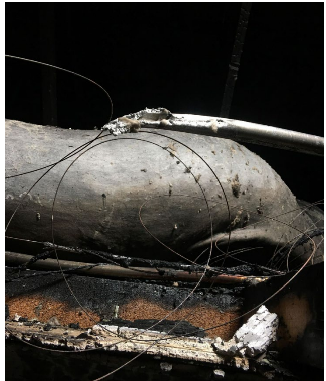
Fire emergency incidents effecting the structural integrity of multilayer pipe leaving open ends allowing uncontrolled gas to escape.
