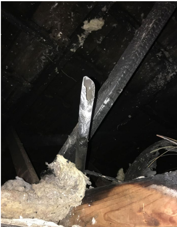
Fire emergency incidents effecting the structural integrity of multilayer pipe leaving open ends allowing uncontrolled gas to escape.
