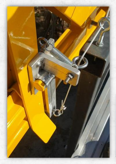
The Void Monitor has been fitted with a fail safe, anti fall, spring return latch, in case the main cable is damaged. This has an additional cable that runs along a separate route, eliminating the risk of the frame from uncontrollably swinging down causing damage or injury.
