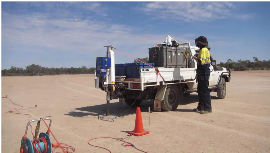
Example of the tow-ball mounted hydraulic ram used to hit a metal plate and generate a small seismic source for active seismic reflection profiling.
