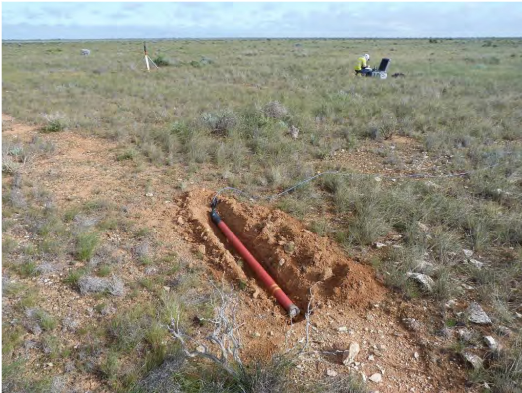
Exmple of a Magnetotelluric deployment. Six shallow holes are dug to bury 4 electrodes and 2 magnetic coils (red tube below). A grey recorder box sits above ground.
