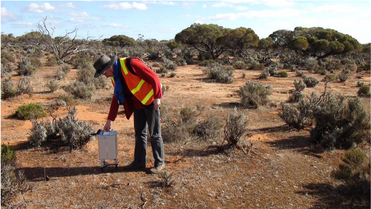
Photo of operator using a gravity meter. There are buttons on the top and a remote control to operate it from a distance.
