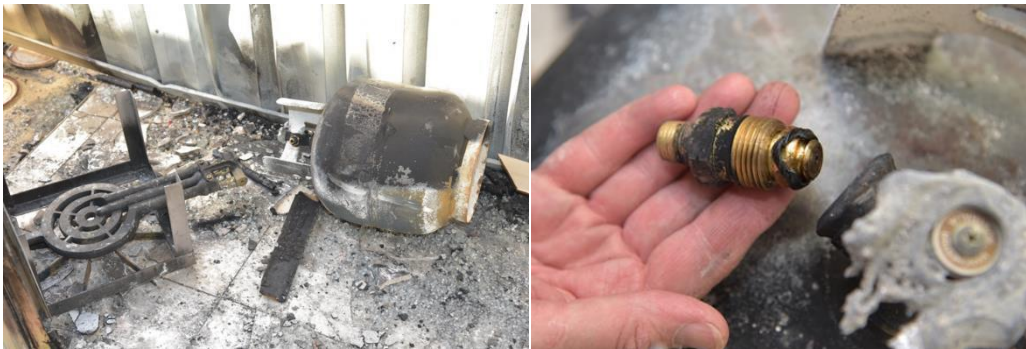
Figure A1 G 21: Outdoor portable wok burner and damaged POL connector involved in explosion incident
