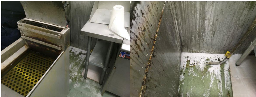
Figure A1 G 19: Deep fryer and open-end hose assembly involved in explosion incident
