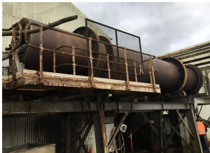
Figure A1 G 18: Rotary salt dryer involved in incident
