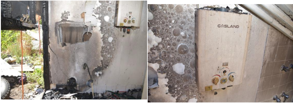
Figure A1 G 20: Recreational outdoor model water heater involved in explosion incident
