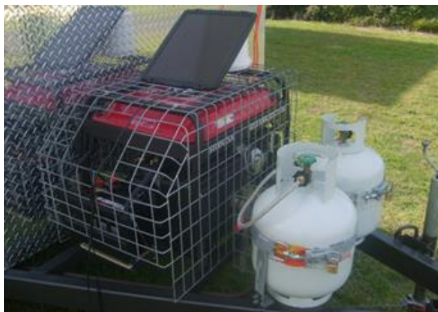
Figure G 9: Example of non-compliant portable generators
