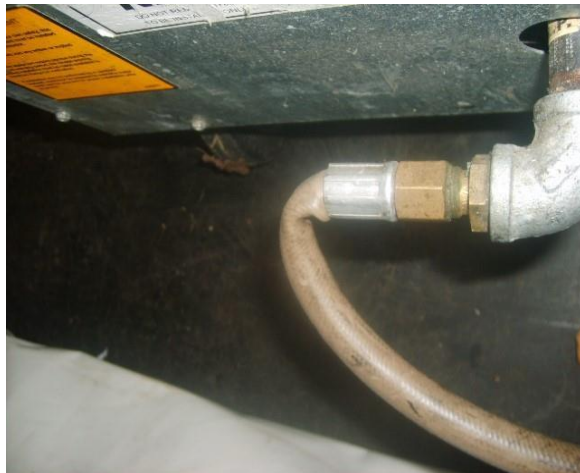
Figure G 8: Example of a damaged gas hose on a temporary cooking setup at an outside event
