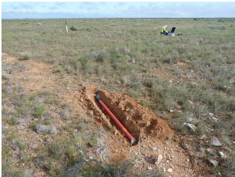
Example of a Magnetotelluric deployment. Six shallow holes are dug to bury 4 electrodes and 2 magnetic coils (red tube above). A grey recorder box sits above ground.
