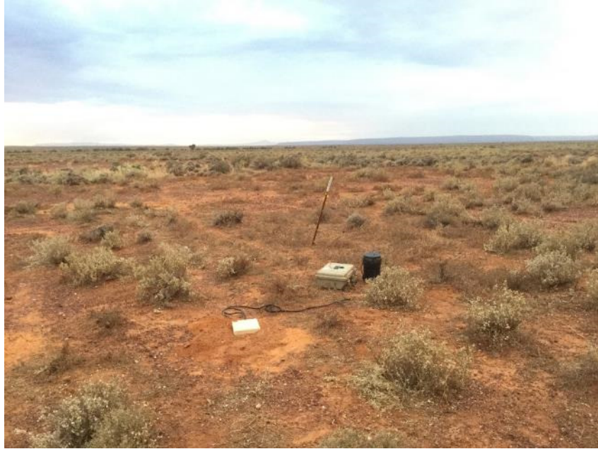
Photo of passive seismic deployment. An auger hole, maximum 50 cm deep contains the seismometer. Battery and recorder are left above ground.
