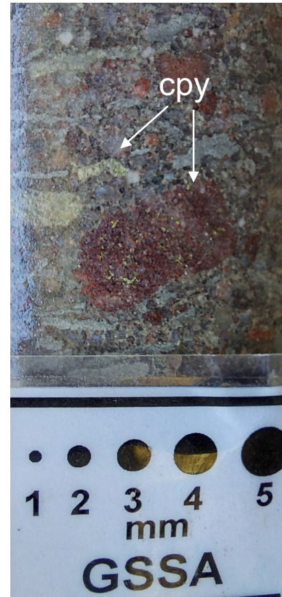
Emmie Bluff – clast and matrix cpy, replacement textures
