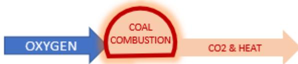
If efficient combustion is sustained, the cavity expands up and out. The main process is still combustion, although transition to gasification develops with growth of the chamber. The exhaust gases heat coal along the flow path, causing pyrolysis that adds gases such as H<sub>2</sub>, CO, CH<sub>4</sub>, C<sub>2</sub>H<sub>4</sub>.
