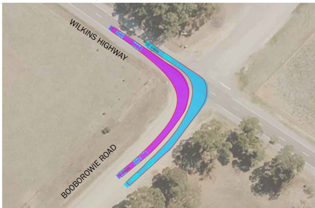
Figure 11 - 19.0 m Semi-Trailer turn paths at the Wilkins Highway/Booborowie Road intersection
