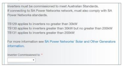
The next section relates to commissioning of a new inverter. Select to which Standard or Technical Standard the inverter has been commissioned to. The required settings will be displayed once you select a Standard. If for some reason the inverter has been commissioned to different settings, select Other and a new section will open for you to enter these details.
