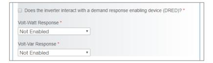
The final section allows you to describe whether the inverter interacts with a demand response enabling device and if the Volt-Watt and Volt-Var modes are enabled.
